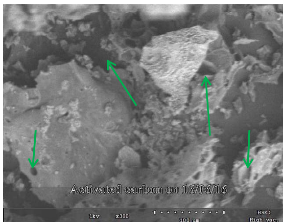
Plate 5: SEM of activated carbon from African star apple seed at x300
