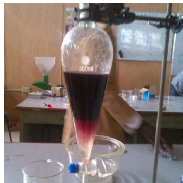
Plate II: Esterified oil in separating funnel
