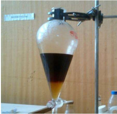
Plate III: Biodiesel in separating funnel
