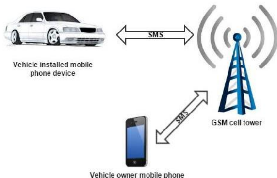
Fig.1. Physical architecture of the theft alert function
