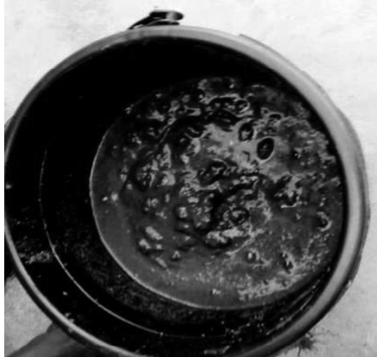
Plate 1: Prepared slurry for feeding into digester
