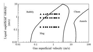
Fig. 11. Flow pattern maps showing the flow patterns determined from PDFs in the present experiments. Vertical case downstream of the contraction. ▲ Bubbly flow; ■ spherical cap bubble; \* transition to slug flow; ● slug flow. The bubble to slug line is from Taitel et al. (1980), that for slug to churn is from Jayanti and Hewitt (1992) and that from churn to annular is from Barnea (1986).
