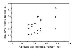
**Fig. 20.** Changes in lengths of liquid slugs and Taylor bubbles across contraction. Inclined case. Closed symbols – upstream; open symbols – downstream. ♦ Liquid slugs; ▲ Taylor bubbles. Upstream liquid superficial velocity = 0.24 m/s.
