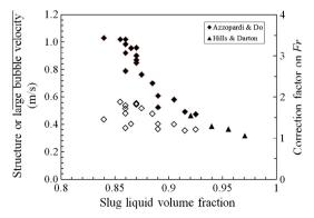
**Fig. 1.** Effect of small bubble in the liquid of velocity of Taylor bubbles. Closed symbols – large bubble velocity; open symbol,  $\diamondsuit$  – correction factor K in Eq. (1). Data from Azzopardi et al. (2014b) and Hills and Darton (1976).
