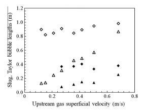
Fig. 18. Changes in lengths of liquid slugs and Taylor bubbles across contraction. Vertical case. Closed symbols – upstream; open symbols – downstream. ♦ Liquid slugs; ▲ Taylor bubbles. Upstream liquid superficial velocity = 0.52 m/s.
