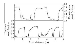
**Fig. 8.** Void fraction time series plotted against axial distance (obtained by multiplying time by structure velocity). Data from upstream (—) and downstream ( $\cdots$ ) of the contraction showing signals typical of slug flow. Inclined case. Upstream gas superficial velocity = 0.49 m/s. Upstream liquid superficial velocity = 0.24 m/s.
