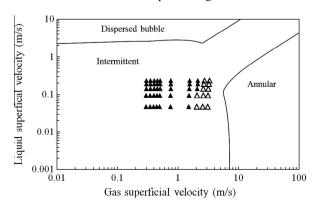
**Fig. 12.** Flow pattern maps showing the flow patterns determined from PDFs in the present experiments. Inclined case upstream of the contraction.  $\blacktriangle$  Slug flow;  $\triangle$  annular flow. The lines are from Shoham (2006).
