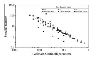
**Fig. 23.** Plot of dimensionless frequency based on gas superficial velocity against Lockhart Martinelli parameter for horizontal pipes and Venturis. 26 mm – Fuklano et al. (1983); 32 mm – Jayanti et al. (1990); 50 mm – Paras and Karabelas (1991); main section – 38 mm diameter – Geraci et al. (2007); throat, modified throat – Geraci (2005).
