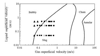
Fig. 10. Flow pattern maps showing the flow patterns determined from PDFs in the present experiments. Vertical case upstream of the contraction. ▲ Bubbly flow; ■ spherical cap bubble; \* transition to slug flow; ● slug flow. The bubble to slug line is from Taitel et al. (1980), that for slug to churn is from Jayanti and Hewitt (1992) and that from churn to annular is from Barnea (1986).
