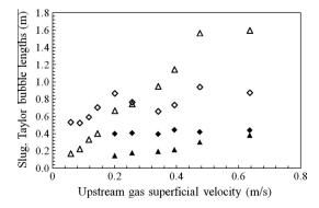
**Fig. 17.** Changes in lengths of liquid slugs and Taylor bubbles across contraction. Vertical case. Closed symbols – upstream; open symbols – downstream. ♦ Liquid slugs; ▲ Taylor bubbles. Upstream liquid superficial velocity = 0.05 m/s.
