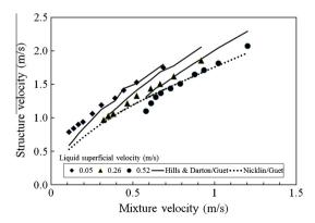
**Fig. 14.** Effect of mixture velocity and liquid superficial velocity on structure velocity (velocity of Taylor bubble, upstream pipe, vertical case. The three solid line correspond to liquid superficial velocities of 0.05, 0.26 and 0.5 m/s, respectively from top to bottom.
