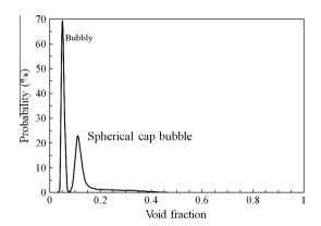
Fig. 5. PDFs of void fraction times series illustrated in Fig. 4.
