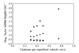
**Fig. 19.** Changes in lengths of liquid slugs and Taylor bubbles across contraction. Inclined case. Closed symbols – upstream; open symbols – downstream. ♦ Liquid slugs; ▲ Taylor bubbles. Upstream liquid superficial velocity = 0.05 m/s.
