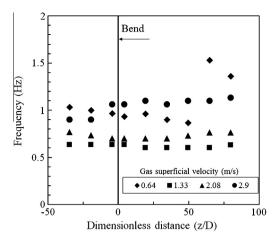
**Fig. 24.** Frequency along the horizontal and vertical pipes either side of the  $90^{\circ}$  bend. Pipe diameter – 34 mm, liquid superficial velocity – 0.81 m/s. Experiments of Saidj et al. (2014).
