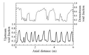
**Fig. 6.** Void fraction time series plotted against axial distance (obtained by multiplying time by structure velocity. Data from upstream (—) and downstream ( $\cdots$ ) of the contraction showing signals typical of slug flow. Vertical case. Upstream gas superficial velocity = 0.34 m/s. Upstream liquid superficial velocity = 0.05 m/s.
