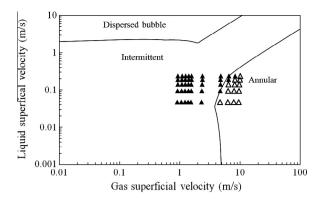
**Fig. 13.** Flow pattern maps showing the flow patterns determined from PDFs in the present experiments. Inclined case upstream of the contraction.  $\blacktriangle$  Slug flow;  $\triangle$  annular flow. The lines are from Shoham (2006).
