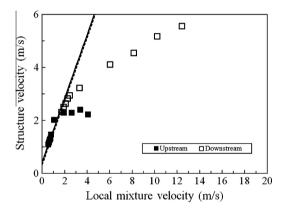
**Fig. 16.** Experimental obtained structure velocities upstream and downstream of the inclined sudden contraction and prediction of form of Eq. (1) [— upstream, ----downstream]. Upstream liquid superficial velocity = 0.24 m/s.
