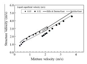
**Fig. 15.** Effect of mixture velocity and liquid superficial velocity on structure velocity (velocity of Taylor bubble, downstream pipe, vertical case. The two solid line correspond to liquid superficial velocities of 0.05 and 0.5 m/s, respectively from top to bottom.
