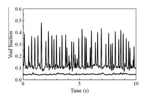
**Fig. 4.** Void fraction times series upstream of the contraction showing signals typical of bubbly and spherical cap bubble flows. Vertical case. Gas superficial velocities = 0.061 and 0.21 m/s, respectively. Liquid superficial velocity = 0.52 m/s.
