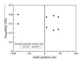
**Fig. 25.** Frequency along the horizontal and vertical pipes either side of the 90° bend. Pipe diameter – 189 mm, pressure – 20 bar – nitrogen/naphtha, Omebere-Iyari and Azzopardi (2007).
