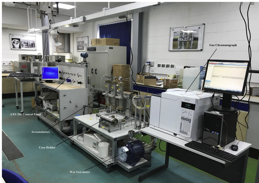
Fig. 3. A perspective depiction of the core flooding setup and the gas chromatograph.
