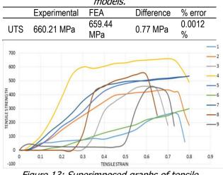
Figure 13: Superimposed graphs of tensile strengths of the 9 weld trials.
