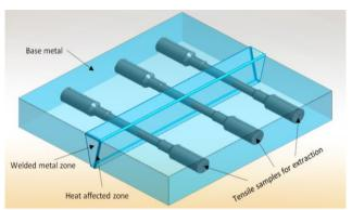
Figure 5: Format for extraction of tensile specimen
