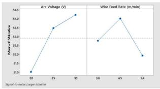
Figure 7: Main effects plot for Tensile strength
