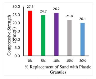
Figure 4: Compressive Strength of Concrete with Plastic Granules Partially Replaced Sand
