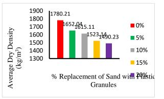
Figure 7: Dry Density of Concrete with Plastic Granules Partially Replaced Sand
