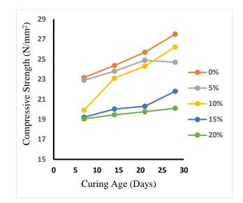
Figure 5: Compressive Strength with Curing age of Concrete with Plastic Granules Partially Replaced Sand.
