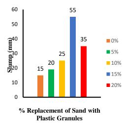
Figure 2: The Slump of Fresh Concrete
