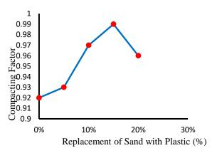
Figure 3: Compacting Factor of Concrete with Plastic Granules Partially Replaced Sand
