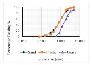
Figure 1: Sieve Analysis for the Aggregates used
