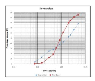
Figure 5: Sieve analysis of Quarry dust and River sand
