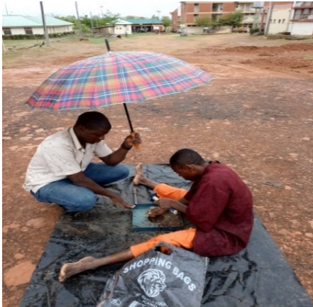
Fig. 10: In-situ density test on the road surface
