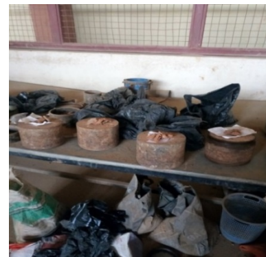
Fig. 4: Compacted samples for CBR test
