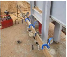
Fig.5: Dial gauges for Settlement Reading
