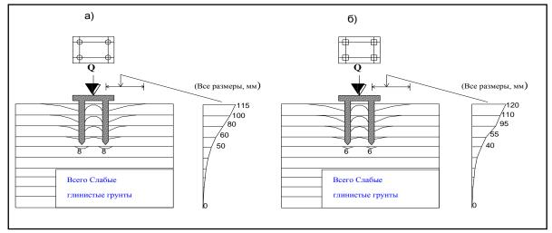
Fig.7: Deformationof2x2-pilegroup for Case-4soil condition:(a) - cylindrical shaped piles (6) tapered conical section.
