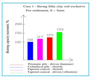
Fig.8: Bearing capacity of piles - case 1
