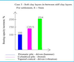
Fig.10: Bearing capacity of piles - case 3
