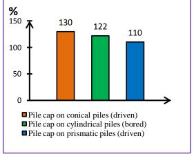
Fig.17: B/Capacity of pile & pile cap - case 5
