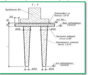
Fig.6: Section of conical shaped pile
