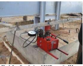
Fig.4: Loading device of 200T capacity HJ
