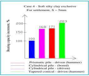
Fig.11: Bearing capacity of piles - case 4
