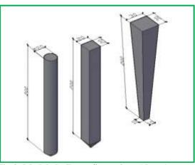
Fig.2: Modeled pile configurations (shape)
