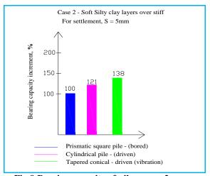
Fig.9:Bearing capacity of piles - case 2
