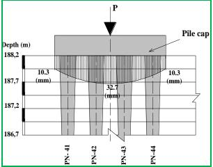
Fig.12: Horizontal Settlement of pile PN-4
