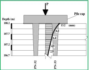
Fig.9: Vertical Settlement of pilePN-1
