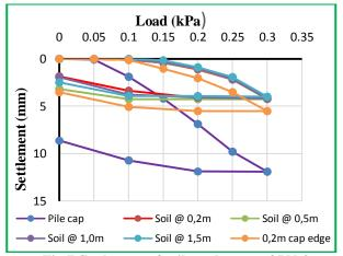
Fig.7:Settlement of soils under cap of PN-3
