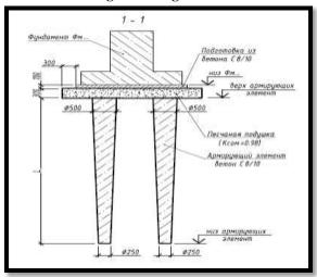
Fig.3:Tapered Piles section on the field
