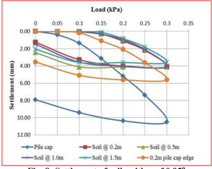
Fig. 8: Settlement of soils with α of 0.95°
