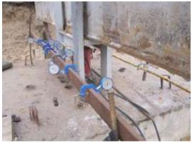
Fig. 4: Dial gauges for Settlement Reading
