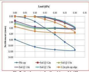
Fig.7: Settlement of soils with α of 1.43°
