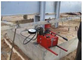
Fig.3: Hydraulic jack for field test loading
