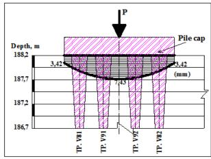
Fig.12: Horizontal Settlement with α of 0.95°
