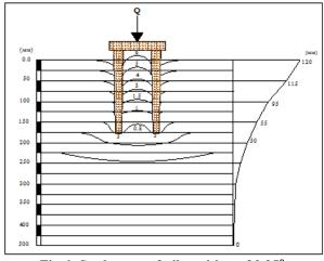
Fig.6: Settlement of piles with α of 0.95°
