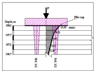
Fig.11: Vertical Settlement with α of 0.95°
