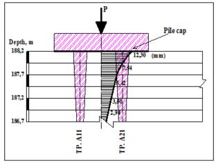
Fig.9: Vertical Settlement with α of 1.43°
