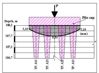
Fig.10: Horizontal Settlement with α of 1.43°
