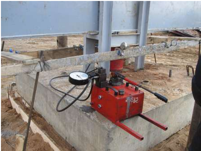
Fig. 1 Hydraulic Jack (200T capacity) for loading
