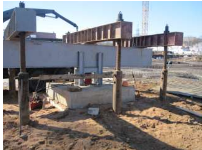
Fig. 2 Full loading assemblage Hydraulic Jack
