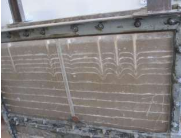
Fig.5 Visual observation of soil displacement under load
