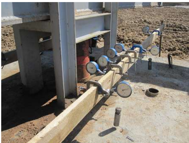
Fig. 1 Hydraulic Jack (200T capacity) for loading
