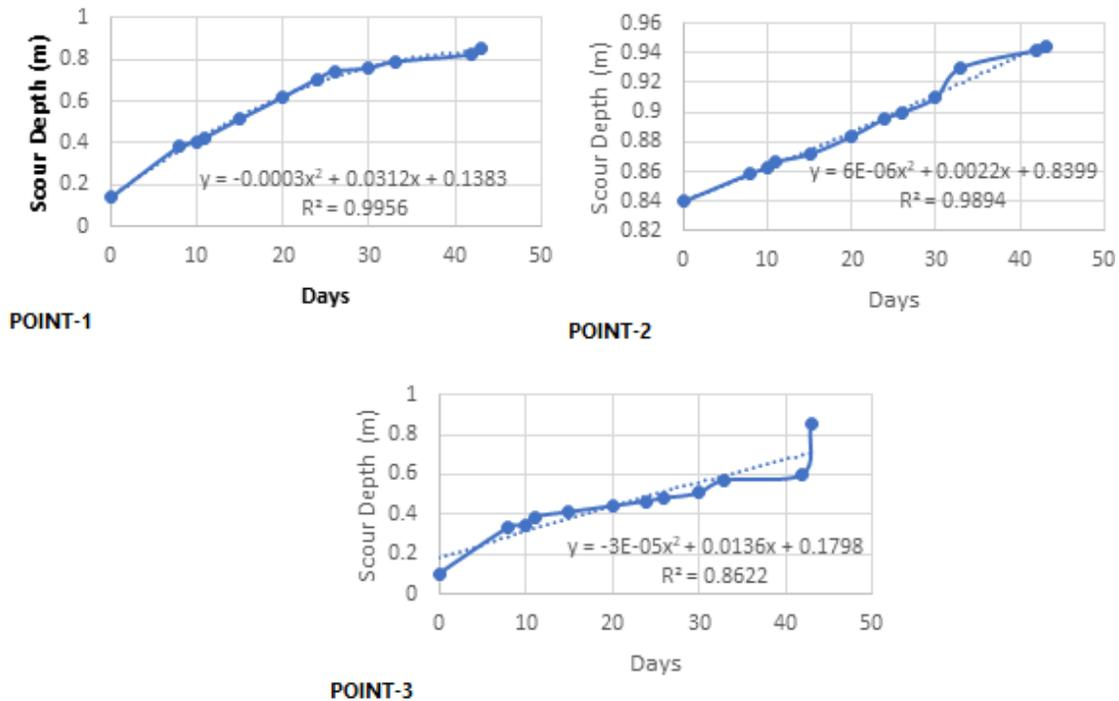
Figure 4. Measured Scour Depth at critical points 1, 2, and 3.
