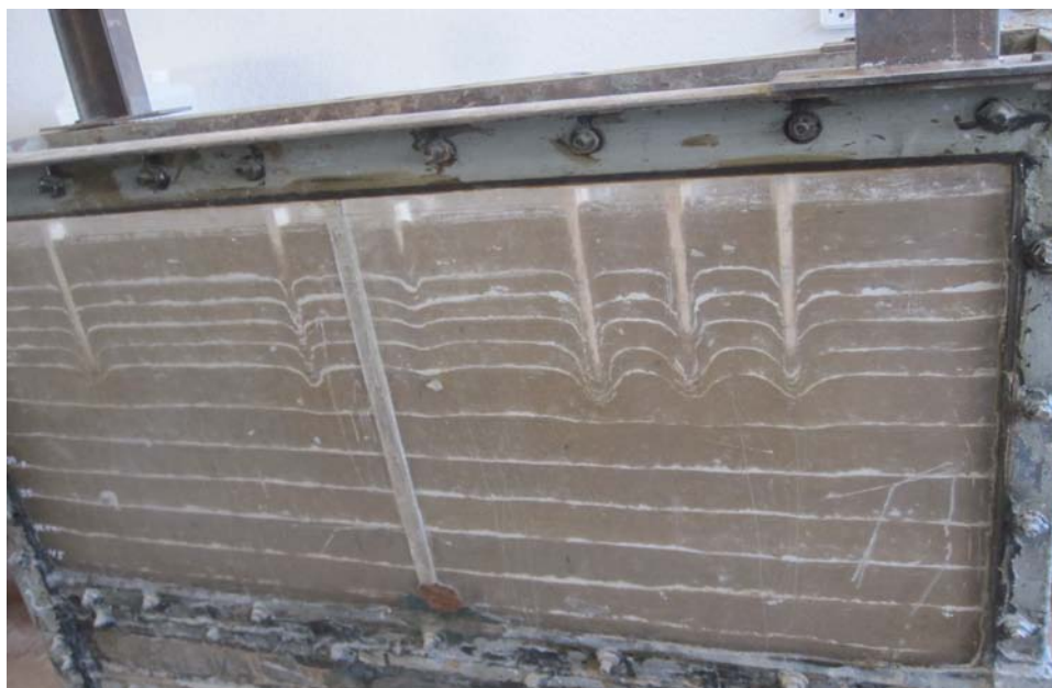
Fig. 8 Testing Tank showing Eaves, Depression and Settlement of Piles
