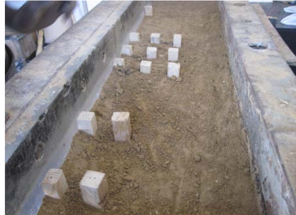
Fig. 2 Pile Driven into Clay in the Tank
