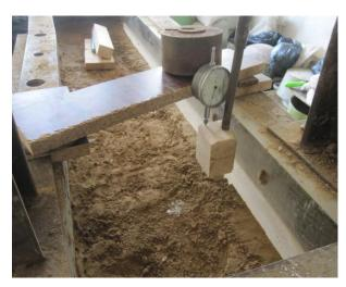
Figure 3. Settlement measurement on Dial gauge
