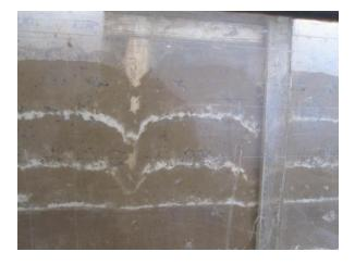
Figure 9. Failure bulb and Deformation Zones under load
