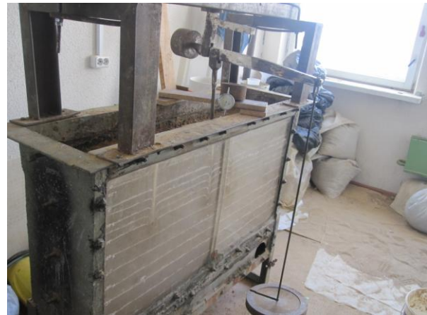
Figure 1. Test tank and load application on the Soil
