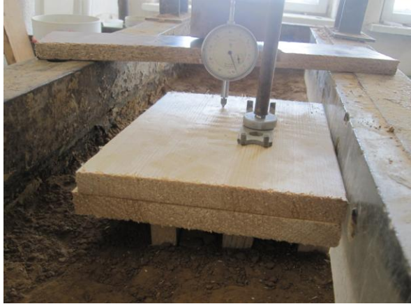
Figure 3. Settlement measurement on the Dial gauge
