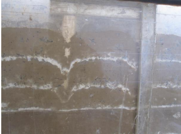
Figure 9. Pressure bulb and Deformation Zones under load
