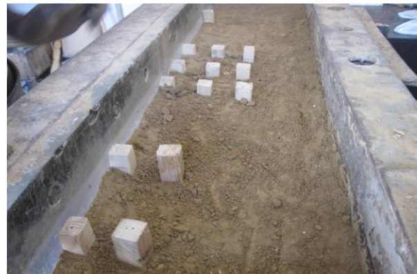
Figure 2. Prototype piles driven into clay in the tank
