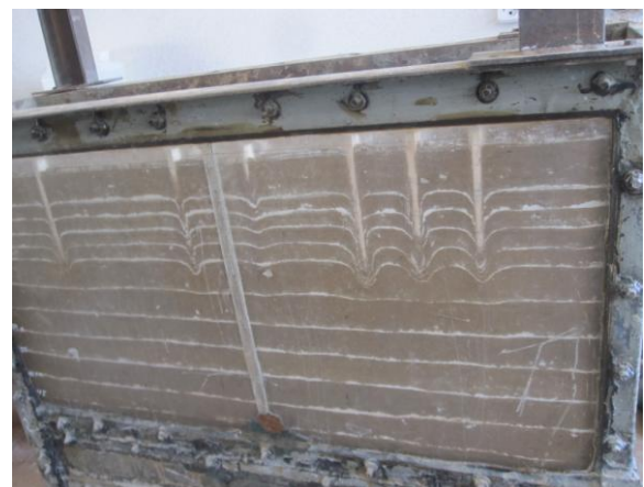
Figure 8. Eaves, depression and settlement of pile
