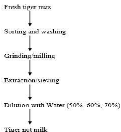
Figure 1: The flow chart for tiger nut milk production
