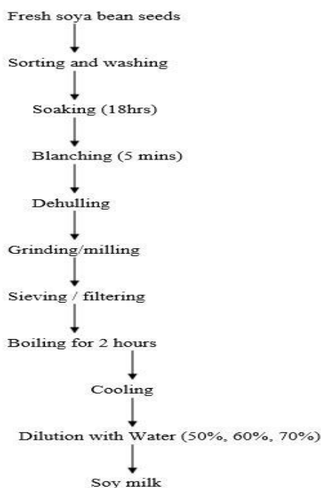
Figure 2: The flow chart for soymilk production
