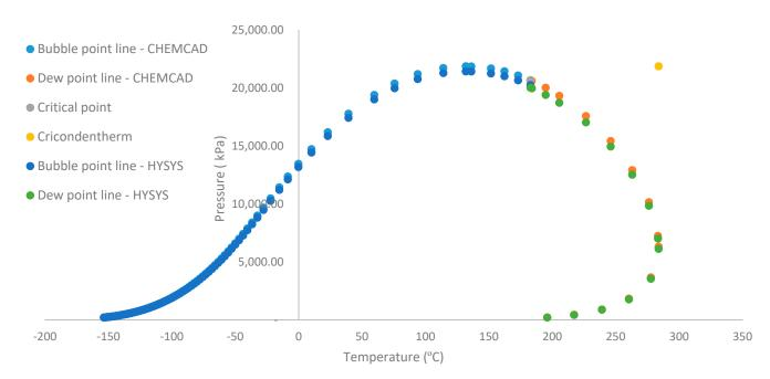
Figure 5. Feed stream phase envelope drawn by HYSYS and CHEMCAD.
