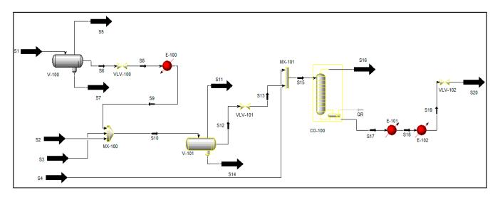
Figure 1. A process flow diagram for the separation process of reservoir fluid developed using HYSYS.
