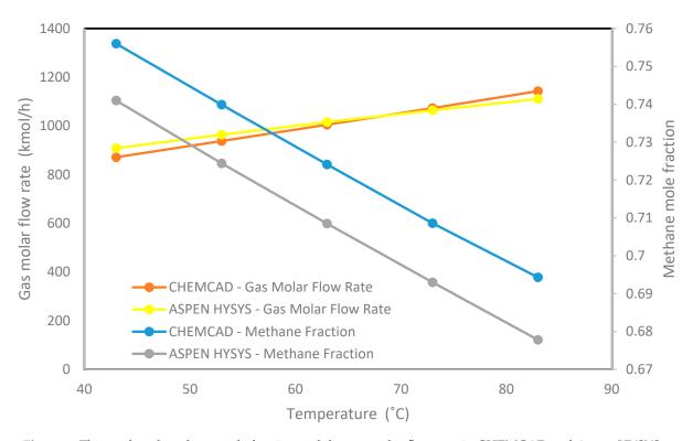
Figure 7. The produced methane mole fraction and the gas molar flow rate in CHEMCAD and Aspen HYSYS.
