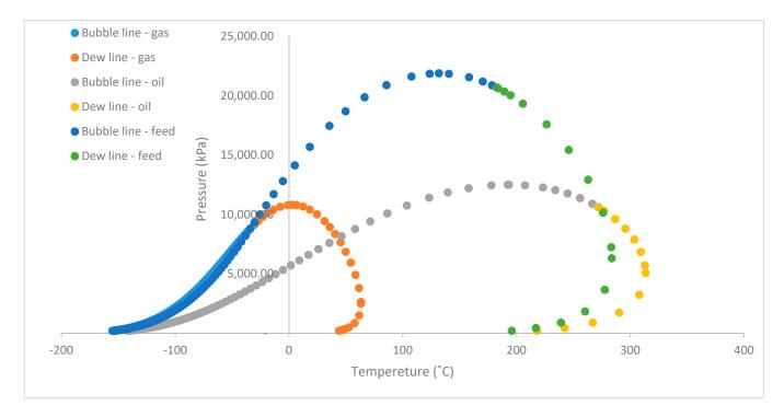
Figure 6. Phase envelopes of feed stream, gas stream, and oil stream obtained from HYSYS.
