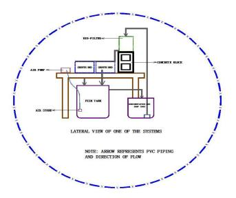
Schematic diagram of the Re-circulatory Aquaponics System
