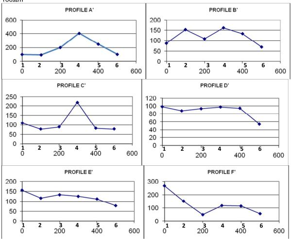
Figure 6: a - f: Wenner configuration ( $\rho$  ( $\Omega m$ ) Vs Distance (m)) for profile A' – F'
