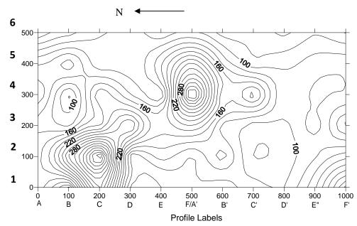
Figure 7: Contour map of Electrical Profiling at 15m Depth (Contour interval is 20**Ωm)**
