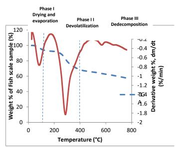
Figure 1: TGA and DTG of Fish scale
