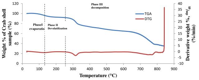
Fig. 1. Thermogravimetric Analysis (TGA) and Derivative Thermogravimetric (DTG)
