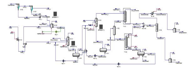
Fig 1: Process Flow Diagram for Bioethanol from Sugarcane Bagasse
