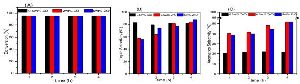
Fig. 5: Aromatic selectivity for the three different ZnO wt% loadings
