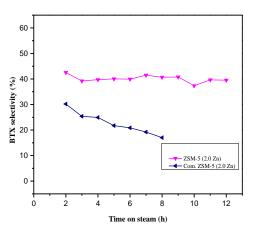
Figure 5 Selectivity of BTX as a function of time on stream.. Reaction conditions: P = 1atm, T = 540 °C, WHSV = 1200 ml/g.h and N2/C3H8 molar ratio = 2.
