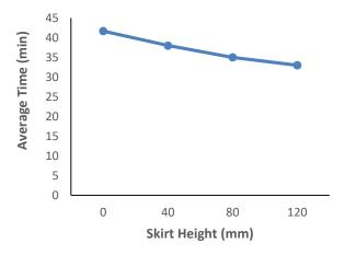
Fig. 3. Graph of the average time (min) taken for the WBT with increasing skirt height (mm)
