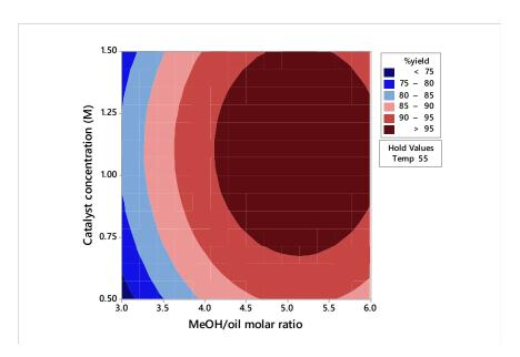
**Fig. 1.** Contour plot showing effect of catalyst concentration and methanol/oil molar ratio on biodiesel yield in transesterification of *L. acida* seed oil.
