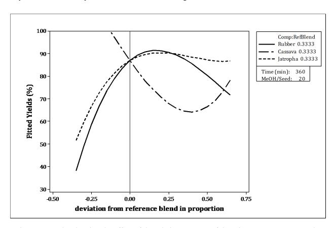
Fig. 1a. Cox plot showing the effect of the relative amounts of the mixture components on the biodiesel yield relative to the reference blend.
