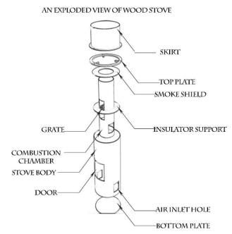
Fig. 1. An exploded diagram of the wood stove
