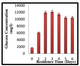
**Figure 3**: Effect of contact time on saccharification at a fixed *A. niger* concentration of 0.6 %( w/v), pH of 4.5, particle size of  $\geq$  125 $\mu$ m, substrate concentration of 50 g/l, and temperature of 30 °C.
