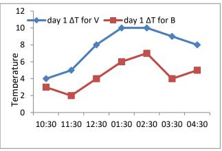
**Fig. 3**. Temperature difference between water and glass against time.
