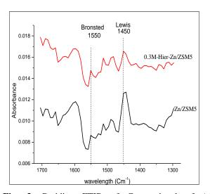
$\begin{tabular}{ll} \textbf{Fig. 3.} & Pyridine & FTIR & of & Conventional & of & (a) \\ & conventional & Zn/ZSM5 & (b) & 0.3M & hierarchical & Zn/ZSM5 \\ \end{tabular}$
