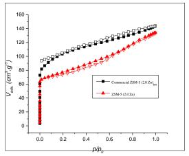
Figure 3:  $N_2$ adsorption-desorption isotherms of Zn/ZSM-5 commercial and Zn-ZSM-5 synthesized samples
