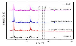
Fig. 1: XRD patterns ZSM-5 (Si/Al=50) and the different ZnO wt% loadings on ZSM-5
