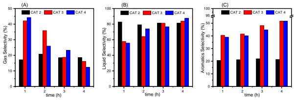
Fig. 5. (A) Gas, (B) Liquid, and (C) Aromatics Selectivity at 520 °C and catalyst: diluent = 50%:50%
