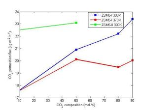
**Fig. 4.**  $CO_2$  permeation fluxes as function of  $CO_2$  feed composition of the ZSM5-I at 300K, 373K and ZSM5-II at 300K under constant feed pressure of 6 bar and permeate pressure of 1 bar.
