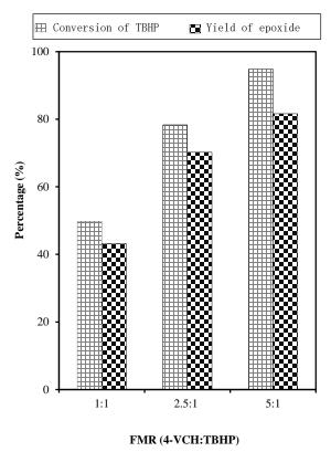
**Fig. 4.** Effect of feed flow rate on the conversion of TBHP and the yield of 4-VCH 1,2-epoxide at steady state for continuous epoxidation of 4-VCH with TBHP using a FlowSyn continuous flow reactor in the presence of Ps.AMP.Mo catalyst (~1.5 g) at reaction temperature: 353 K; feed molar ratio of alkene to TBHP: 5:1.
