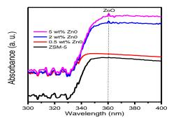
Fig. 2: UV-Vis spectra of the catalysts, with ZSM-5 (50) as reference
