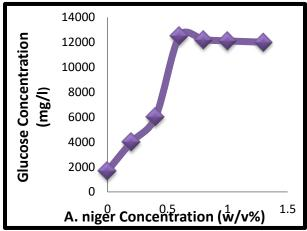
Figure 5: Effect of *A. Niger* Concentration on Saccharification at a fixed pH of 4.5, residence time of two (2) days, particle size of  $\leq 125 \mu m$ , substrate concentration of 50 g/l, and temperature of 30 °C
