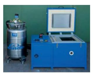
Fig. 1: Set-up of cryogenic treatment in the temperature of 77 – 450 K, which consists of a well-insulated treatment chamber (right), liquid nitrogen in a Dewar vacuum flask (left), (Linde gas, sub-zero treatment of steels, technology/processes/equipment).
