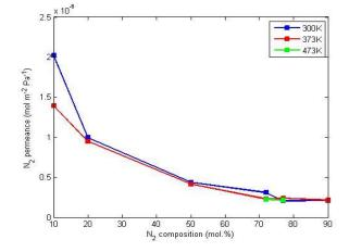
**Fig. 3.**  $N_2$  permeances as function of  $N_2$  feed compositions at 300K, 373K and 473K and constant feed and permeate pressures of 6 bar and 1 bar respectively.
