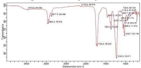
Fig. 4: FTIR of H<sub>2</sub>SO<sub>4</sub>-catalyzed butyl acetate.
