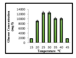
**Figure 2:** Effect of temperature on saccharification at *A. niger* concentration of 0.6% (w/v), pH of 4.5, particle size of  $\leq 125$  µm, substrate concentration of 50 g/l, and residence time of two (2) days.
