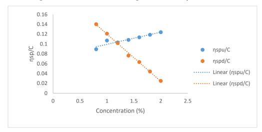
Fig 3: Viscosity of dyed and undyed starch paste.
