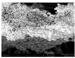
**Plate 1.** SEM for tamarind starch
