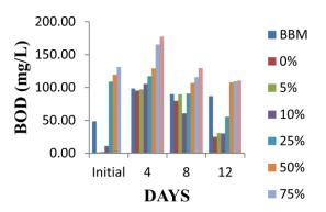
Fig. 1 Effect of *Chlorella vulgaris* on Biological Oxygen Demand (mg/l) at different dilutions treated tannery effluent
