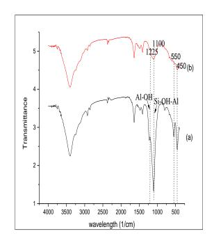
**Fig. 2.** FTIR patterns of (a) Conventional Zn/ZSM5 (b) 0.3M hierarchical Zn/ZSM5
