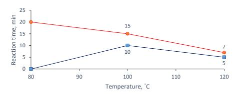
Fig. 2: Relationship between the reaction time for the esterification and temperature.
