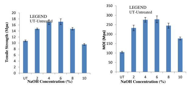
Fig. 1 and 2: Effect of Fibre Treatment on the Tensile Strength and Modulus of Elasticity of the Baobab/Sisal Hybrid Composite
