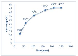
**Fig. 3:** Moisture loss for stage wise drying of *blended onions*
