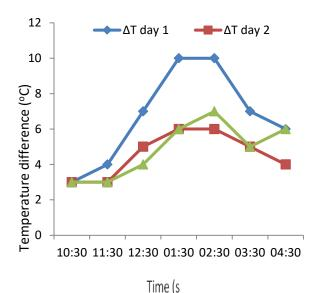
**Fig. 1.** Temperature difference between water and glass for day 1, 2 and 3.
