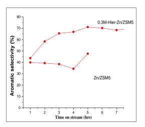
**Fig. 6.** Aromatic selectivity over Conventional & hierarchical Zn/ZSM5 catalysts
