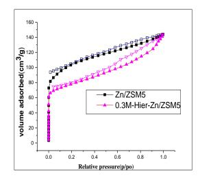
**Fig. 4.** Nitrogen adsorption–desorption isotherms of conventional and 0.3M-hierarchical Zn/ZSM5 samples at 77k
