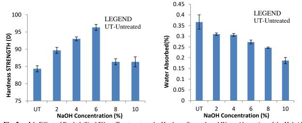
Fig. 5 and 6: Effect of Baobab/Sisal Fibres Treatment on the Hardness Strength and Water Absorption of the Hybrid Composite
