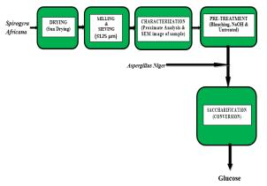
Figure 1: Block Diagram Showing the Method for Glucose Production from *Spirogyra africana*
