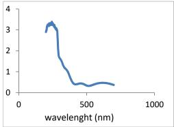
Figure 4: UV spectrum for Fe(II) complex
