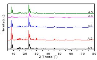
Figure 1: XRD pattern of ZSM-5 Si/Al =50; (A1) conventional ZSM-5, (A2) acid treated ZSM-5, (A3) 0.3wt% iron loading on ZSM-5, (A4) 0.6 iron loading on ZSM-5, and (A5) 1wt% iron loading on ZSM-5
