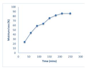
**Fig. 1**: Moisture loss for straight drying of sliced onions at (95°C)
