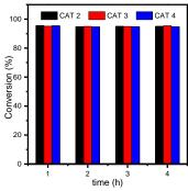
**Fig. 4.** LPG conversion at 520  $^{\circ}$ C and catalyst: diluent = 50%:50%
