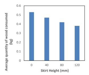
**Fig. 2.** Bar chart of average quantity of wood consumed (kg) for the WBT for the stove and skirts with increasing heights (mm)
