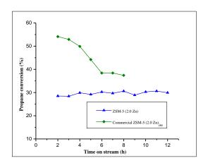
Figure 4: Propane conversion as a function of time on stream. Reaction conditions: 1atm, 540 °C, WHSV of 1200 ml/g.h and N2 to C<sub>3</sub>H<sub>8</sub> molar ratio of 2.
