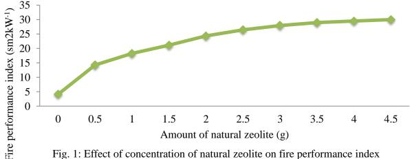
Fig. 1: Effect of concentration of natural zeolite on fire performance index (FPI) of the intumescent flame retardant PVC sheets
