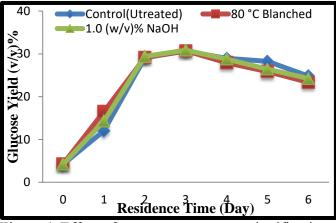
Figure 4: Effect of pre-treatment on saccharification at following hydrolysis conditions: temperature 30 °C, pH 4.5, substrate concentration 50 g/L, *A. niger* concentration 0.65 % (w/v), and particle size  $\leq$  125  $\mu$ m.
