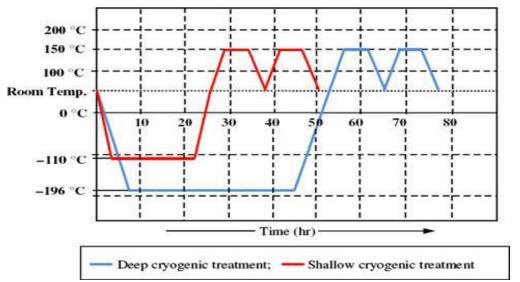
Fig. 2. Time Vs temperature for shallow cryogenic & deep cryogenic treatment (Gill et al., 2011).
