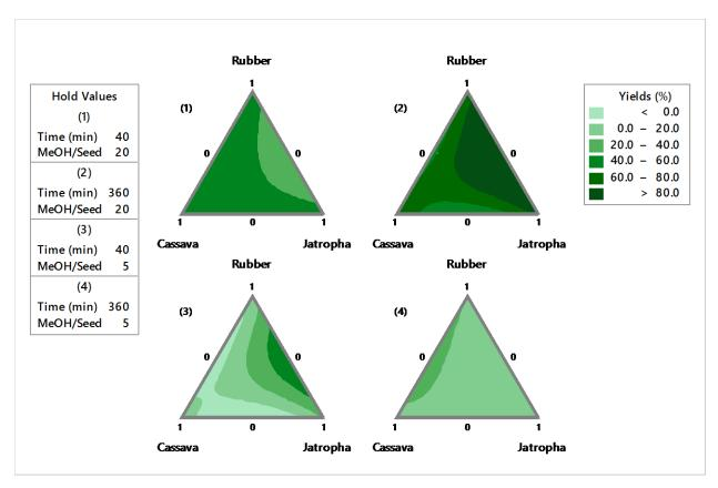
Fig. 1b. Contour plots showing the effect of the mixture components are process variables on biodiesel yield.
