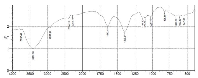
Figure 1: FTIR analysis of the pectin extracted from Adansonia digitata L. pulp.
