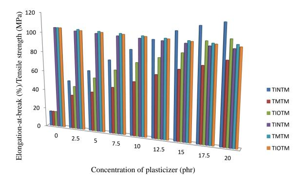
**Fig. 3.** Effect of concentration of TINTM, TIOTM and TMTM on elongation-at-break and tensile strength of the PVC sheets
