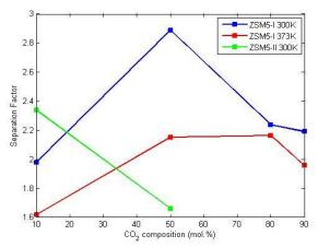
**Fig. 1:** Separation factors as function of  $CO_2:N_2$  feed ratio at 300K and 373K under constant feed pressure of 6 bar and permeate pressure of 1 bar.
