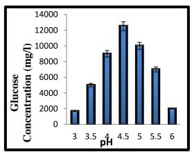
**Figure 4**: Effect of pH on saccharification at a fixed *A. niger* concentration of 0.6 % ( w/v), contact time of two (2) days, particle size  $\leq 125\mu m$ , substrate concentration of 50g/l, and temperature of 30 °C
