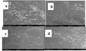
Plate 1: SEM Micrograph of (a) 50:50 untreated, (b) 4 wt% NaOH, (c) 6 wt% NaOH and (d) 10 wt% NaOH treated hybrid sisal: baobab fibre hybrid composite.
