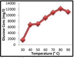
Figure 2: Effect of Blanching Temperature on Glucose Production at the following hydrolysis conditions: temperature 30  $^{\circ}$ C, pH 4.5, substrate concentration 50 g/L, *A. niger* concentration 0.65 % (w/v), and particle size  $\leq$  125  $\mu$ m.
