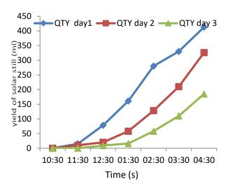
**Fig. 2.** Commulative distillate at hour interval between 10:30 am to 4:30 pm for day 1, 2, and 3 respectively.
