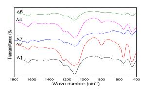
Figure 2: FTIR spectra of ZSM-5 Si/Al=50; (A<sub>1</sub>) conventional ZSM-5, (A<sub>2</sub>) acid treated ZSM-5, (A<sub>3</sub>) 0.3wt% iron loading on ZSM-5, (A<sub>4</sub>) 0.6 iron loading on ZSM-5 and (A<sub>5</sub>) 1wt% iron loading on ZSM-5.
