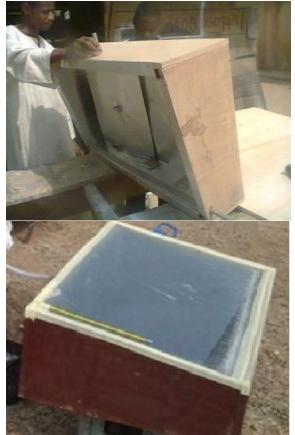
Plate 1. Showing submerged flat plate Plate 2. Showing the solar still
