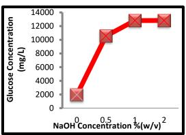
Figure 3: Effect of NaOH Concentration on Glucose Production at following hydrolysis conditions: temperature 30 °C, pH 4.5, substrate concentration 50 g/L, *A. niger* concentration 0.65 % (w/v), and particle size  $\leq 125 \ \mu m$ .
