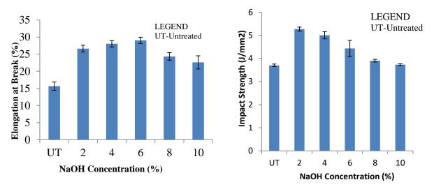
Fig. 3 and 4: Effect of Baobab/Sisal Fibre Treatment on the Elongation at Break and Impact Strength of the Hybrid Composite
