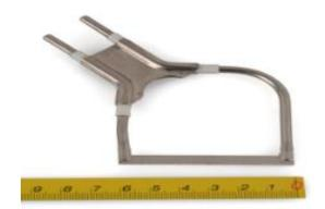
Fig. 3. Cryogenic treated garment cutting knives.
