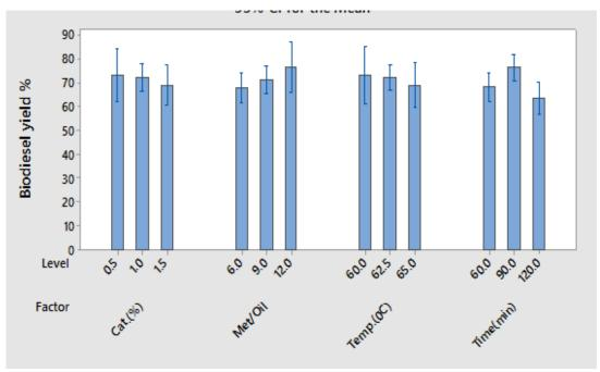
Fig. 1. Summary of the effect of the process variables on the biodiesel yield from neem seed oil.
