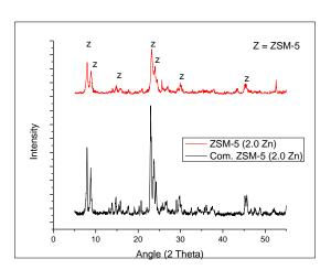
Figure 1: XRD diffraction patterns of commercial and synthesized samples
