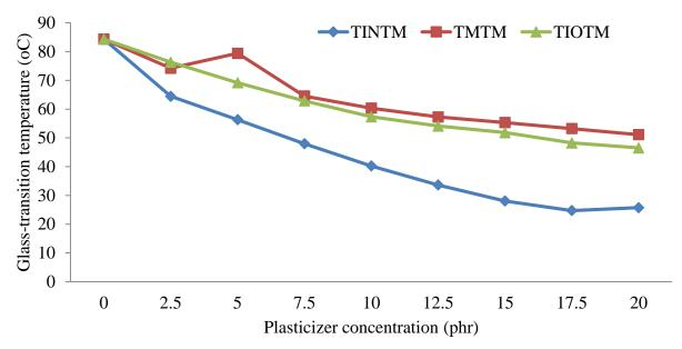
**Fig. 1.** Effect of concentration of TINTM, TIOTM and TMTM on the glass-transition temperature of PVC sheets.
