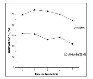
**Fig. 5.** Propane conversion over conventional and hierarchical Zn/ZSM5 samples
