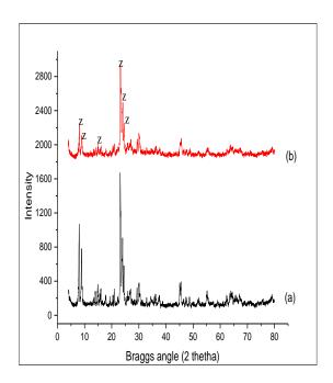
**Fig. 1.** XRD diffraction patterns of (a) conventional Zn/ZSM5. (b)0.3M hierarchical Zn/ZSM5
