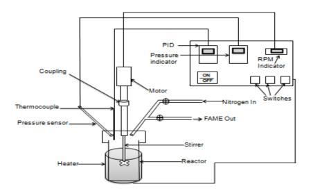
Fig. 1: Schematic diagram of the hydrothermal liquefaction reactor used
