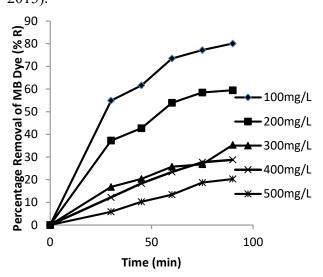
Figure 1: Effect of initial Dye Concentration on Percentage Removal of MB at Different Times
