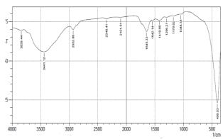
Fig. 3: FT-IR Spectrum of Fe(II) Complex
