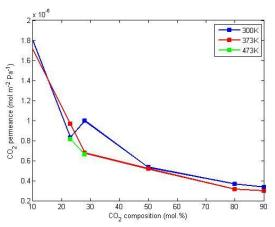
**Fig. 2**: CO<sub>2</sub> permeances as function of CO<sub>2</sub> feed compositions at 300K, 373K and 473K and constant feed and permeate pressures of 6 bar and 1 bar respectively.
