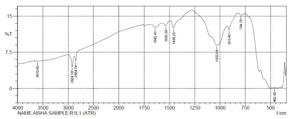
Figure 1: FTIR spectra of the pyrolysis oil sample.
