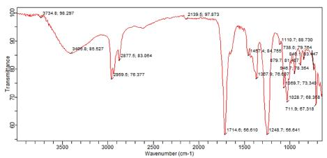
Fig. 3: FTIR of DES-catalyzed butyl acetate.
