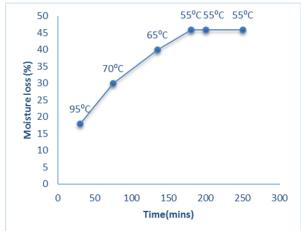
Fig. 2: Moisture loss for stage wise drying of sliced onions
