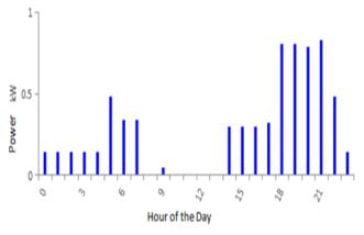
Figure 6. Primary load profile with DSM strategies implemented
