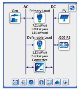
Figure 5. Schematic hybid energy system with DSM strategies implemented
