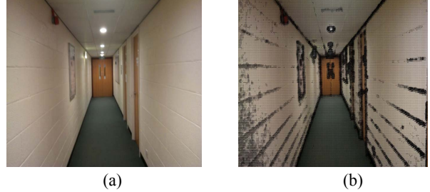
Fig 2. (a) Corridor of a building captured with camera phone (b) The optical flow computed along the corridor of building in (a).
