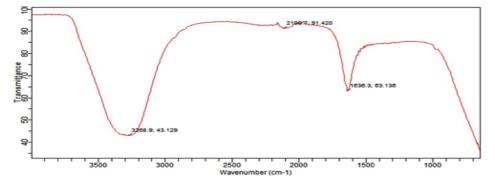
Figure 4: FTIR spectrum of the biosynthesized AgNPs using aqueous stem bark extract of A. *occidentale*.
