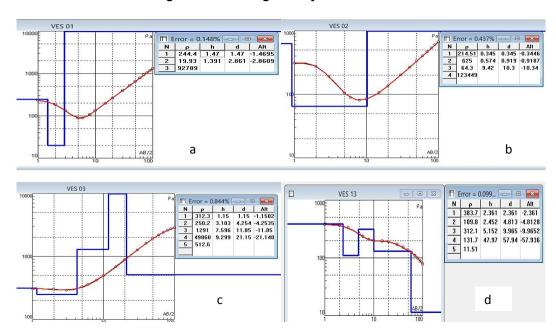
Fig. 8. Typical (a) H-Type curve, (b) HA - Type curve (c) and (d) other 5 - layer curve types
