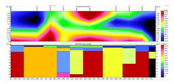
Fig. 13. Pseudo cross-section and Resistivity cross-section of Profile 5 in the study area
