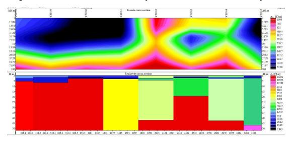
Fig. 14 Pseudo cross-section and Resistivity cross-section of Profile 6 in the study area
