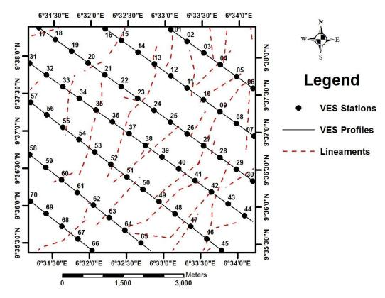
Fig. 2. VES sounding stations along 7 Profiles (Profiles 1 to 7 from top to bottom). The spacing between VES sounding stations are 500 m apart.
