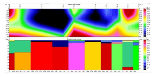
Fig. 12. Pseudo cross-section and Resistivity cross-section of Profile 4 in the study area
