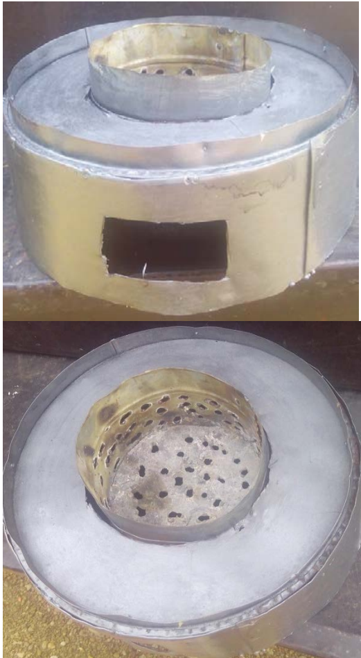
Plate III: Picture of the briquette pot
