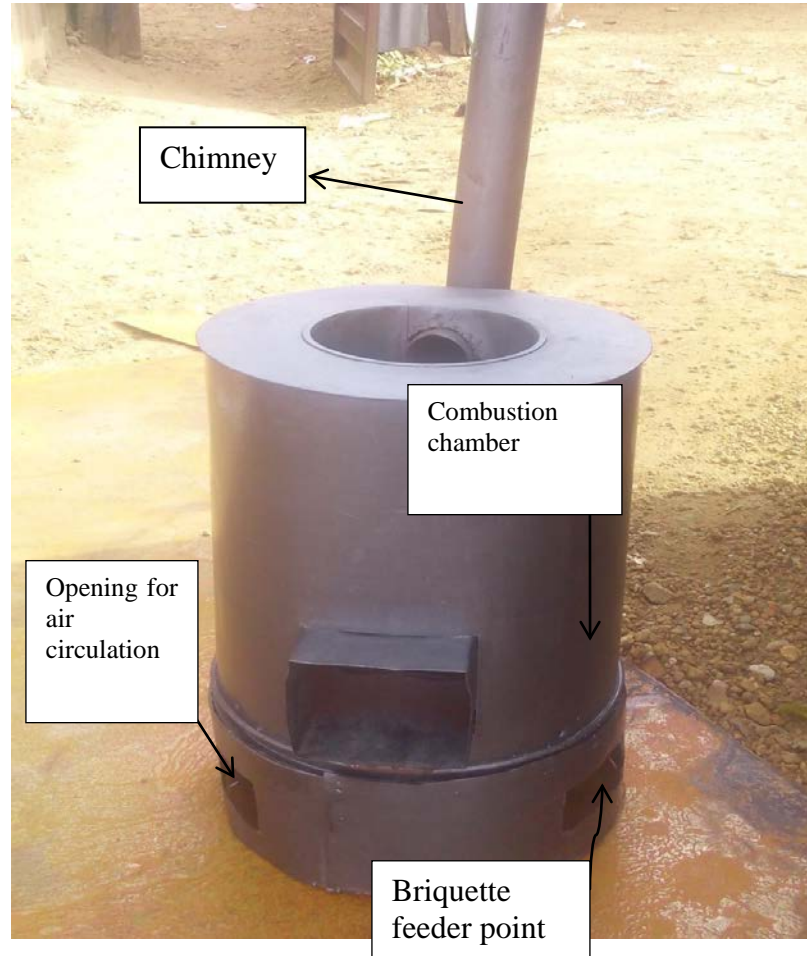
Plate IV: Complete setup of the briquette stove
