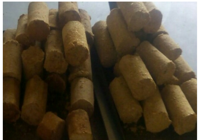
Plate V: Briquettes used for testing the stove
