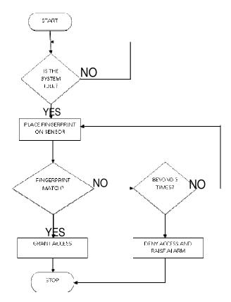
Fig. 3.3: Flow chart design of fingerprint access control system
