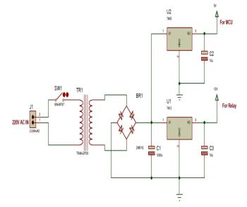
Fig 3.2: Regulated power supply unit
