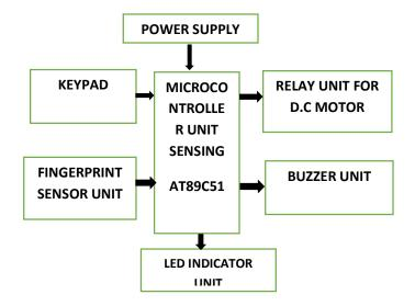
Figure 3.1: Block diagram of the design of fingerprint access control system
