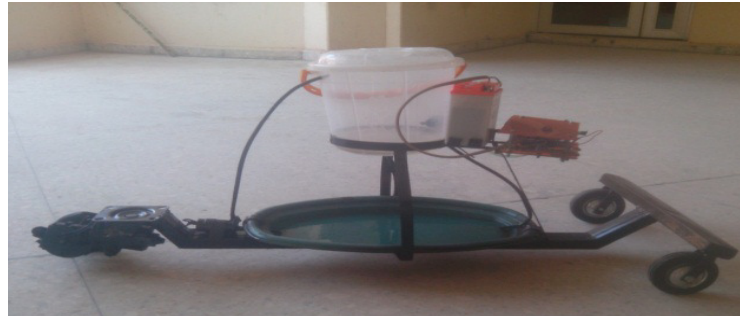
Figure 5: The final developed mobile intelligent liquid feed dispensing system
