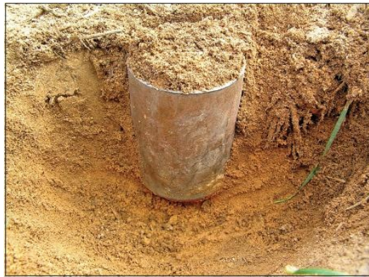
Plate 2: Excavated soil, ready to be oven dried.
