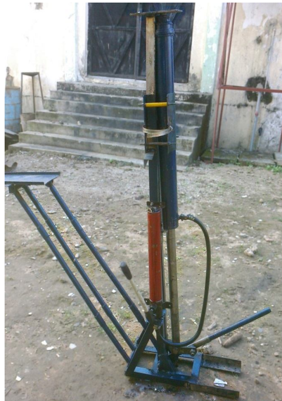
Figure 1. Assembled Hydraulic accumulator lift machine
