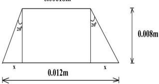
Figure 3: Cross-Sectional Area of the Belt.
