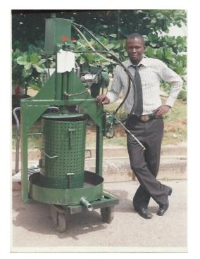
Figure 3: Designed and Fabricated Motorized Hydraulically Operated Palm Oil Press with the Designer Beside it.
