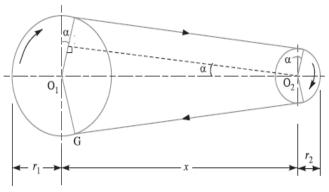
Figure 2: Arrangement of the pulleys. (Source: Khurmi and Gupta 2006)
