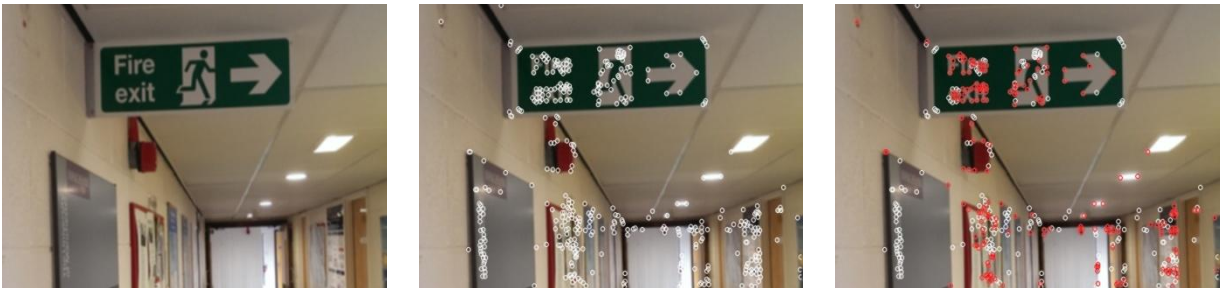
Figure 4.1 (a) Original image showing an exit sign along a corridor of the Kilburn building of the University of Manchester. (b) Keypoints detected using FAST detector. The white circles indicate keypoints that also include other interest points such as edges. (c) In this Image, the red circles show the strongest corner returned after applying a corner response function to the detected feature from AST
