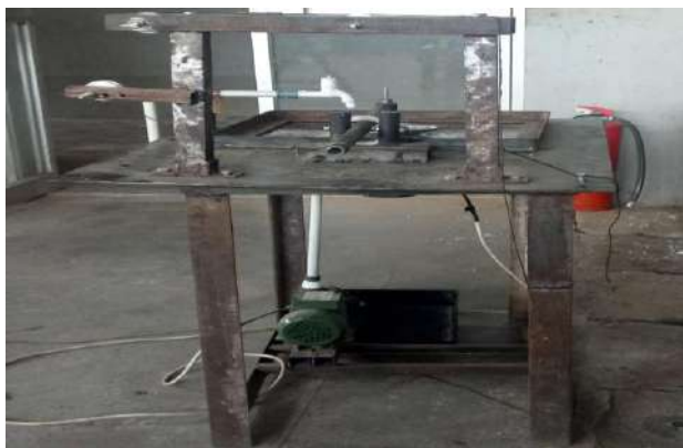
Figure 1: Dual Condition Pin-On-Disc Wear Testing Machine
