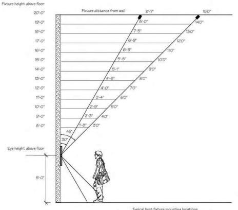
Typical light fixture mounting locations To avoid glare aiming angle should be between 30° and 45°
