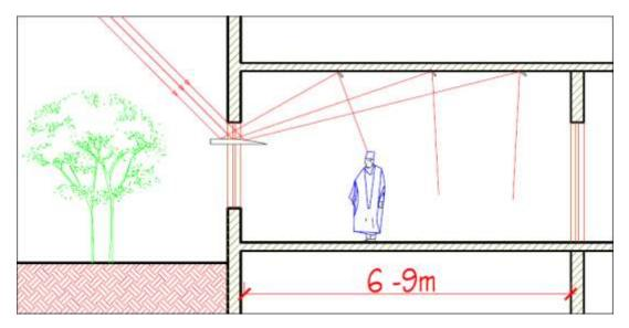
Fig 2.13: How light entering a building can be controlled through the principle of light redirection. (Source: Architect' Data, 2000)
