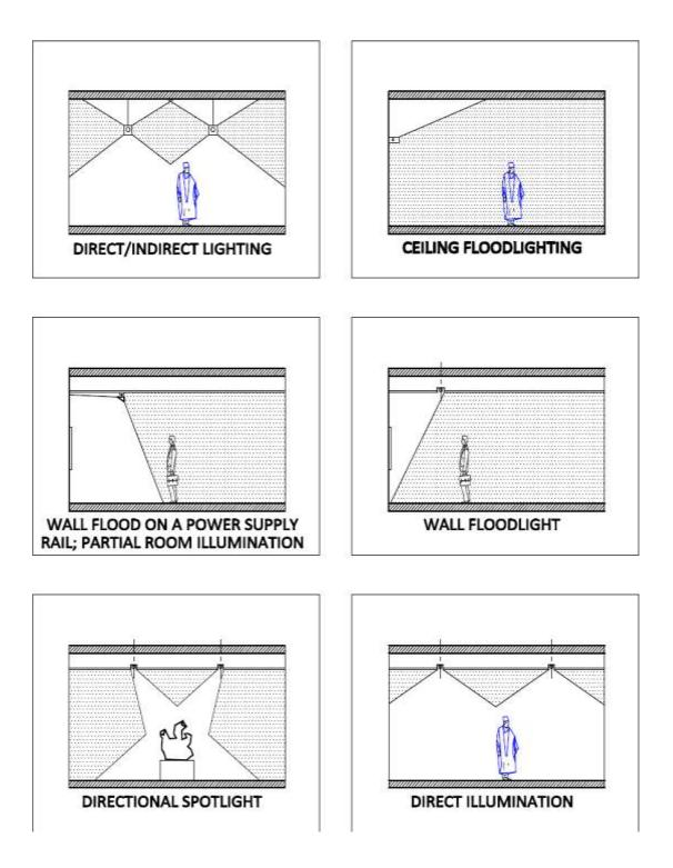
Figure 2.10: The use of various lighting schemes from artificial light sources. (Source: Architect' Data, 2000)
