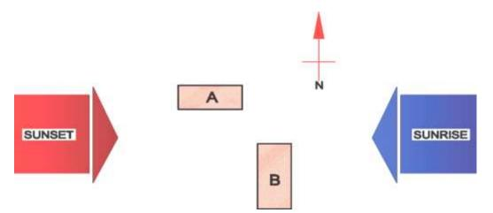
Figure 2.12: How light entering a building can be controlled by proper building orientation, where fewer windows are exposed to the Eastern and Western axis.
