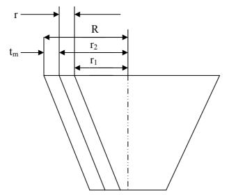
$$S_{t} = \omega^{2} r_{2} \left[ r_{2} \rho_{m} + \left( r_{2}^{2} - r_{1}^{2} \right) \frac{\rho_{c}}{4t_{m}} \right]$$
