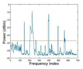
(b) Threshold Using Optimized FCME algorithm
