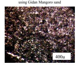
Plate 2. Micrograph of etched Aluminium test sample
