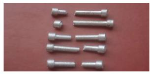
Plate I: Alumiunm Cast Samples after Tensile Tests
