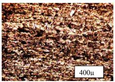
Plate 3. Micrograph of etched Aluminum test sample using Tagwai Dam sand
