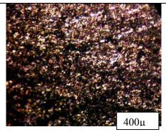
Plate 1. Micrograph of etched Aluminium test sample
