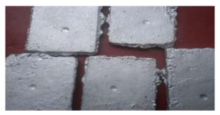
Plate II: Aluminium Cast Samples showing Indention of Hardness Tests
