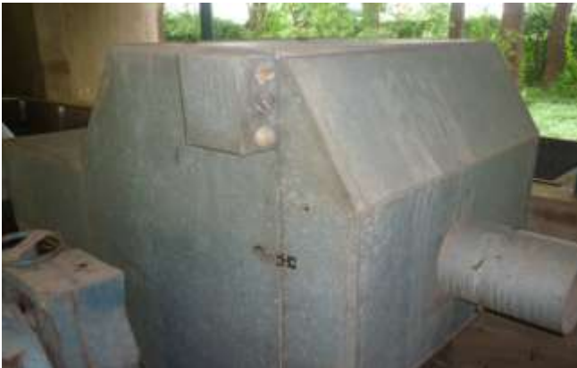
Fig. 10: Platform Sugar Dryer
