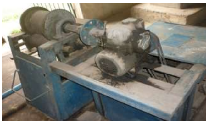
Fig. 3: Roller Juice Extractor
