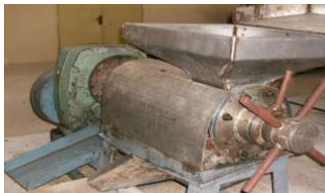
Fig. 5: Cane Juice Expeller
