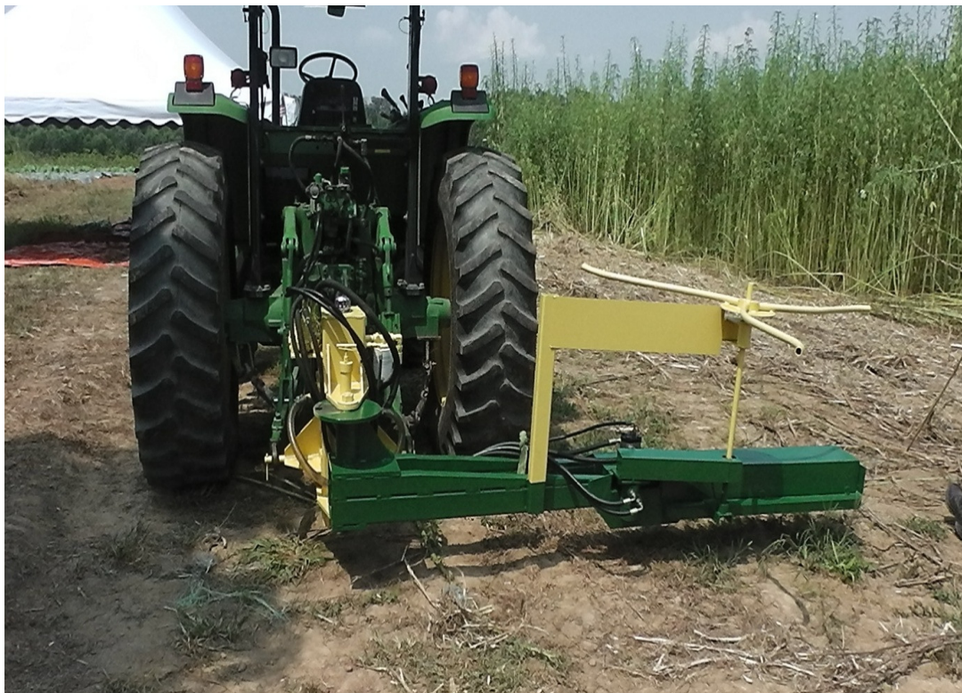
Figure 2. Developed kenaf harvester mounted on a tractor
