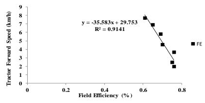
Fig. 5: Effect of speed on field efficiency
