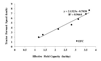
Fig. 4: Effect of speed on effective field capacity
