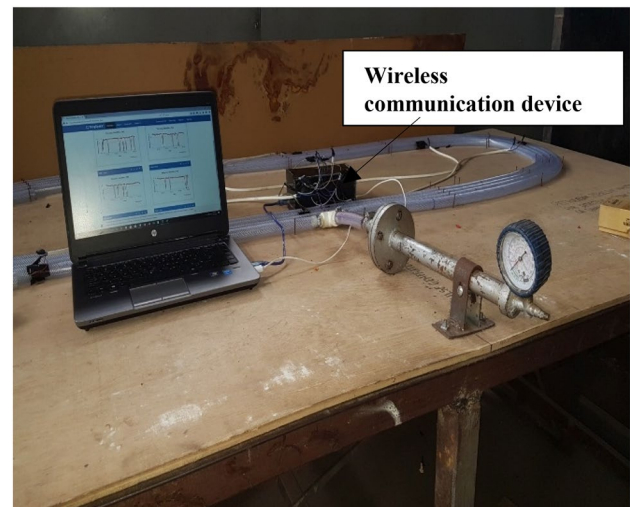
Fig. 5 Experimental test rig 2 with wireless communication device
