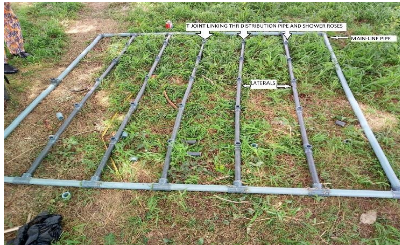
Figure 1: Development of Rain Simulator in Progress
