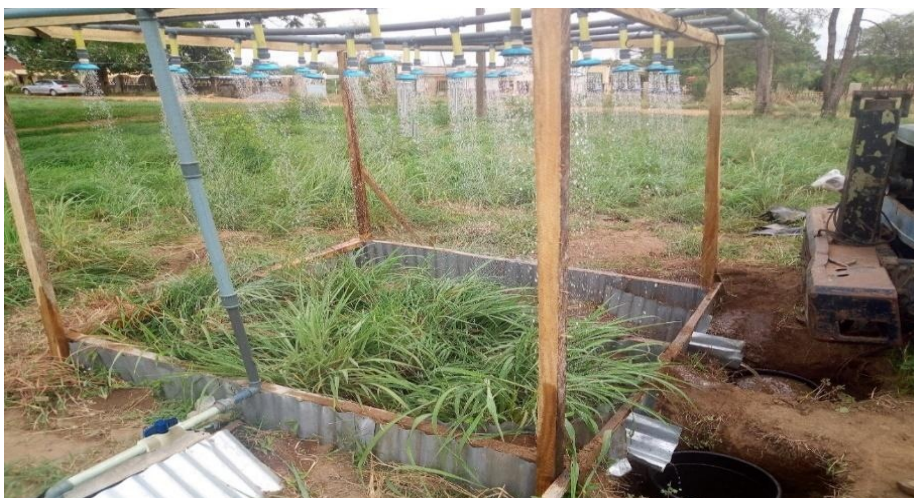
Figure 4: Rainfall simulator in operation
