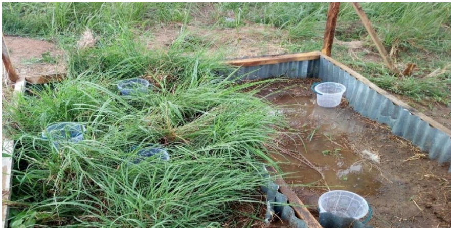
Figure 5: Buckets randomly placed under the simulator for determination of uniformity coefficient
