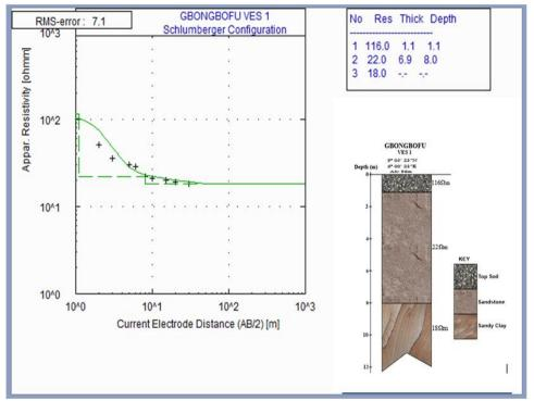
Figure 5: Vertical Electrical Sounding Curve at Gbongbofu Gully Erosion Site
