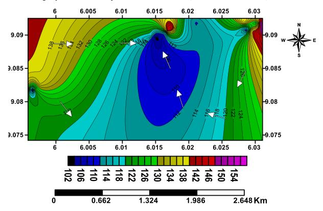
Figure 3: Groundwater flow direction
