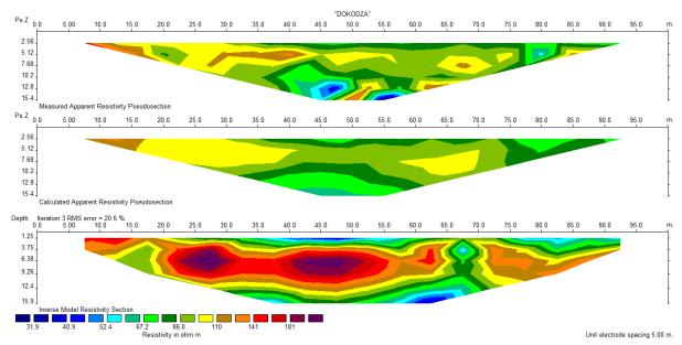
Figure 6: 2D Transverse at Dokoza Gully Erosion Site
