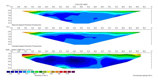
Figure 7: 2D Transverse at Low-Cost Gully Erosion Site in Bida Town
