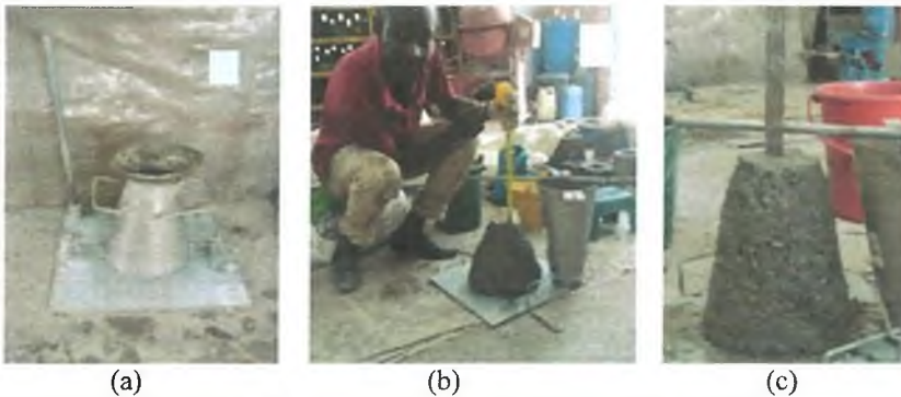
Figure 2 An operational procedures for slump test: (a) Abrams slump apparatus, (b and c) Measurement of slump
