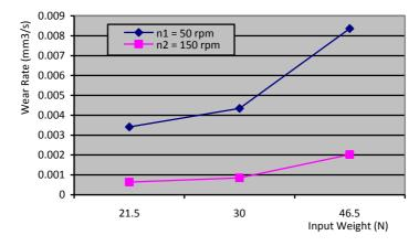
Fig. 3: Effect of input weight on wear rate at D = 200m
