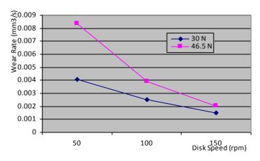
Fig. 4: Wear rate with rotating disk speed at D = 200m
