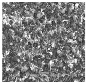
Fig. 1: Micrograph of the *Ti-6Al-4V* surface
