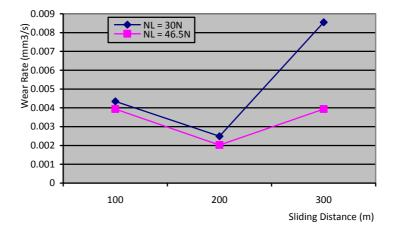
Fig. 5: Wear rate with sliding distance at V = 100 rpm
