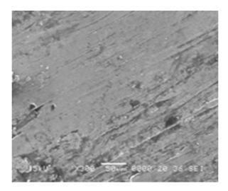
Fig. 2: SEM micrograph of a worn surface (3.00kg, 150rpm)
