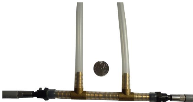
Figure 3 Gas cell of 10.8 cm optical path length that consists of two equal T brass gas connectors that are jointed together using silicone tubes. Gas cell is connected to collimating lens, optical fibers, ozone gas inlet and outlet. Size of gas cell is compared to Malaysian 10 cent coin
