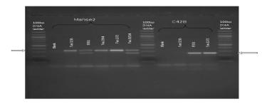
Fig. 4. PCR amplification of DNA based on the use of BIONEER Accupower PCR premix with the SCAR(marker Mahse2 and C42B) in 2% agarose gel with ethidium bromide staining.
