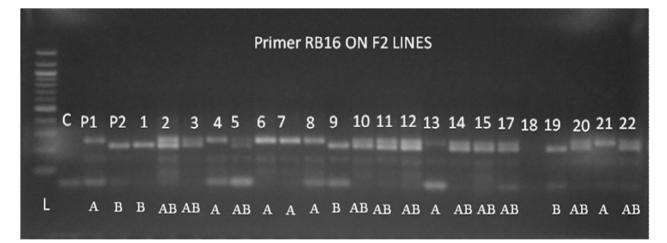
Plate 2: Sample image of agarose gel electrophoretic analysis of PCR amplified product using primer RB16 for the F2 progenies derived from B301 x Banjar. L = 100 bp ladder, C =control without genomic DNA template. P1 = B301, P2 = Banjar.
