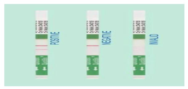
Figure 1: Cry1Ab/1Ac Bt strips showing positive, negative and invalid result (Envirologix, 2008)
