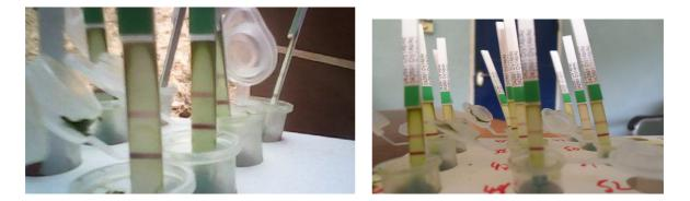
Figure 2: Cry1Ab/1Ac Bt strips in test tubes showing positive results (Field Result 2012)
